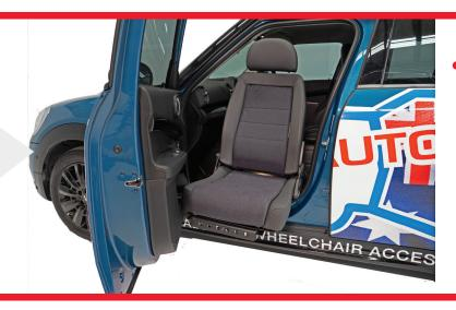
Convenient safe solution for easy access to vehicles with higher seating positions. Allowing the car seat to rotate out through the door opening and lower to a suitable height for transfer to and from the vehicle.
