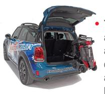
These enable you to lift a mobility device, such as a wheelchair, scooter or powerchair, easily and quickly into your car boot at the touch of a button.
